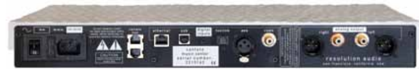
All the usual digital inputs, but also an Ethernet port.
